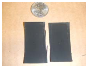
Figure 4. Carbon cloth electrode material after being sprayed
