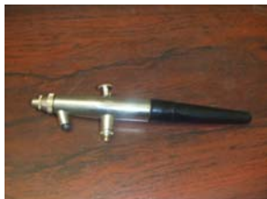
Figure 3. Airbrush used for spraying technique
