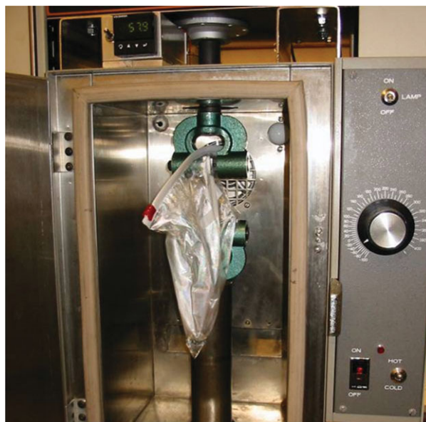
Figure 1. Instron 1122 and environmental chamber used for stress–strain tests. The plastic bag vapor barrier was installed to for elevated humidity tests. [Color figure can be viewed in the online issue, which is available at www.interscience.wiley.com .]
